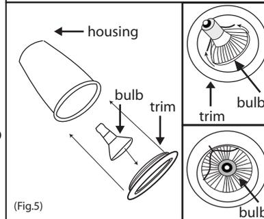
5. Install the proper bulb - Max 50 w GU10 Shielded and Canarm Trim as specified above. (Fig.5)
