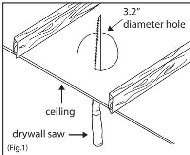
1. Using 3.2" template on the box, mark the openings and cut the openings with a drywall saw where you intend to install the lights. (Fig.1)
